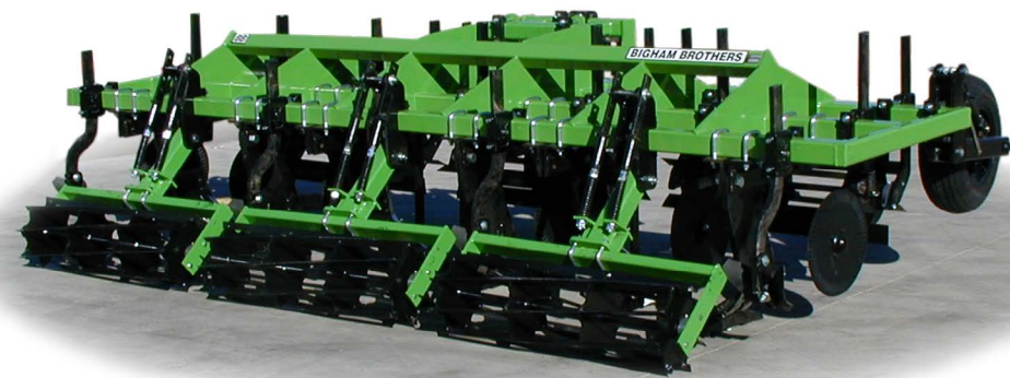
Parabolic Ripper. 4x7" Front, Double 4x4" Rear.
