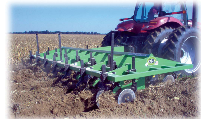
One Pass TerraTill® for Corn. 4x7" Front and Rear, Triple 4x4" Center.
