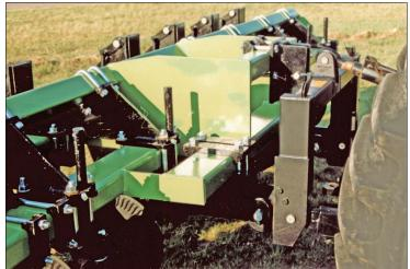
Heavy duty diamond mast frame has 4 x 7 x 3/8" tube on all lower frame members. Optional extended front hitch mount provides flexibility to place coulters and Legs on any row spacing. Heavy Category III Wide 4" Drop Hitch is standard on all models.
