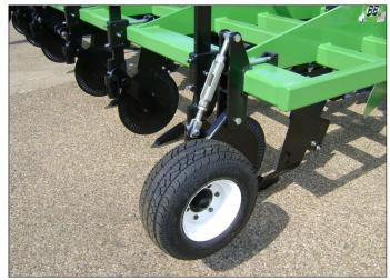
Heavy duty diamond mast frame has 4 x 7 x 3/8" tube on all lower frame members. Optional extended front hitch mount provides flexibility to place coulters and Legs on any row spacing. Heavy Category III Wide 4" Drop Hitch is standard on all models.
