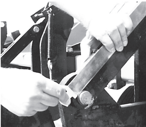
Picture 7: Seat lower portion of measuring tool on lower pin.
