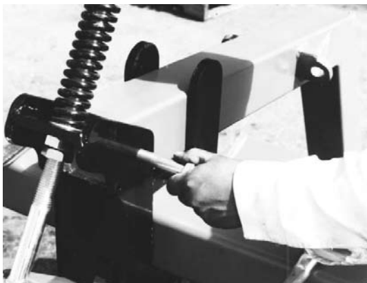
Picture 19: Insert bolt through roller arm.
