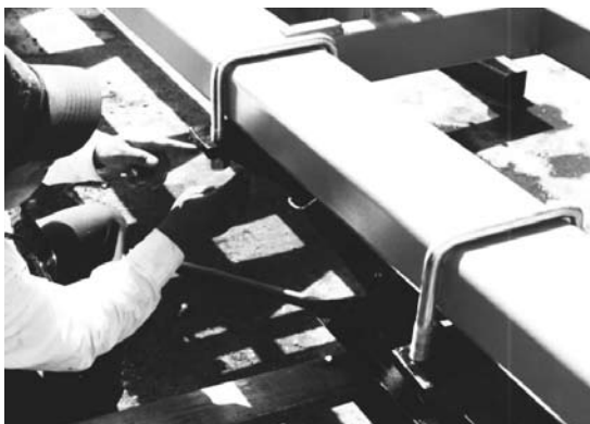
Picture 14: Place U-bolts on tool bar to mount chopper.
