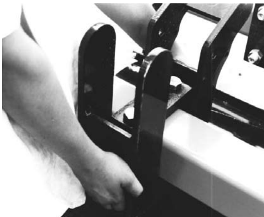
Picture 15: Raise mount bracket and fasten nuts.
