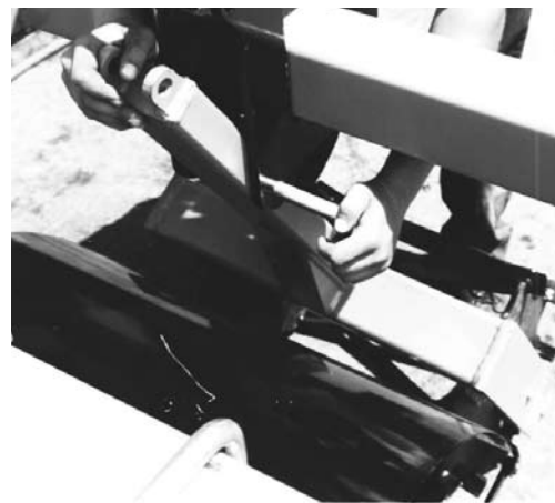
Picture 16: Insert bolt through pivot arm.
