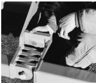
Picture 5 - Remove hinge shipping tab from front hinge.
