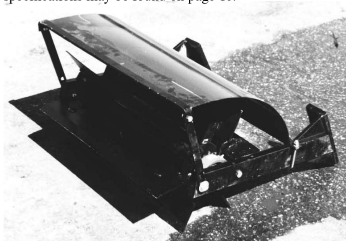
Picture 12- Sub-assemble chopper before attaching to tool bar.
