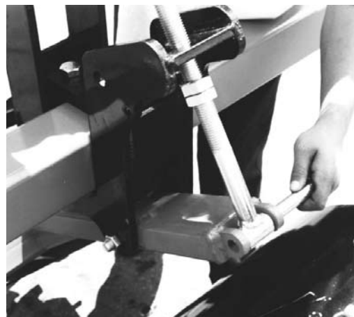
Picture 17: Insert bolt through yoke and screw jack bushing
