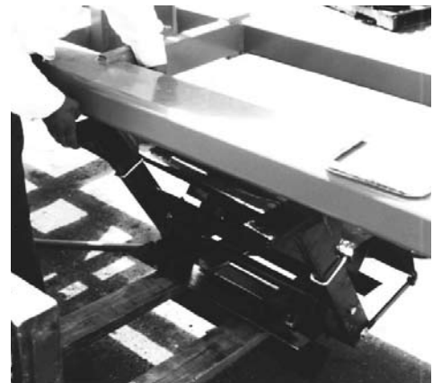
Picture 13- Position chopper to mount on the front bar.
