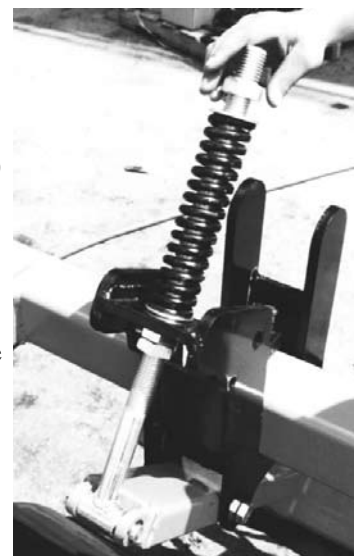
Picture 18: Complete upper spring assembly.
