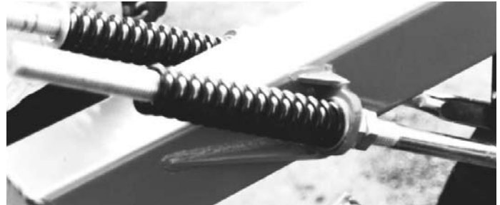
Picture 21: Complete rear spring assembly.
