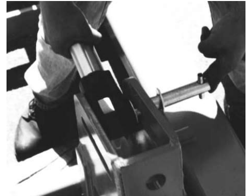
Picture 9 - Insert wing lift pin.
