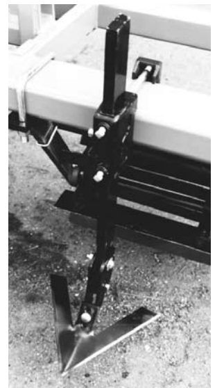
Picture 22: Stalk plow shank on front tube.
