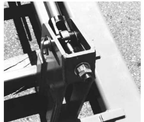
Picture 10 - Wing lug has been assembled.
