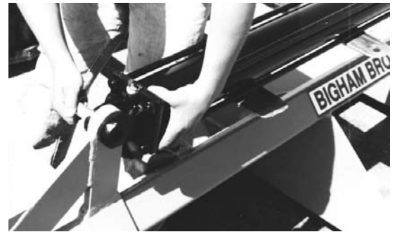
Picture 8 - Install cylinder base pin.
