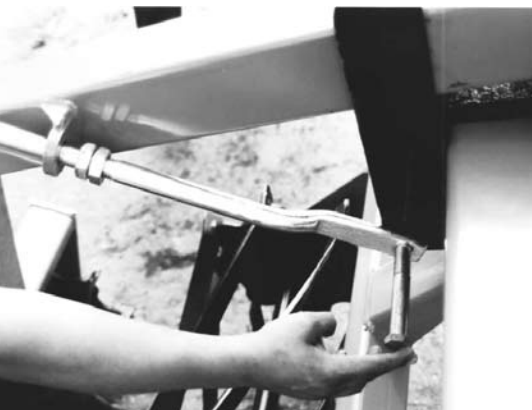
Picture 20: Insert bolt through spring rod lug.
