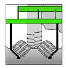
TerraTill® loosens a more narrow zone to allow maintenance of a firm traffic lane in row spaces from 30" to 32". TerraTill® fits well with narrow row cotton (particularly on a stale seedbed) as well as corn, milo soybeans and other crops traditionally produced on narrow rows.
