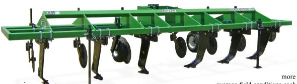
Break up compaction without destroying soil structure. The Bigham TerraTill® bends subsoil to remove hardpans. The TerraTill® uses the same leg design principles that makes the Paratill successful, but provides a narrower, more shallow loosened zone. In
