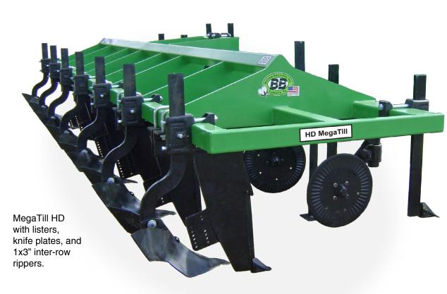
The MegaTill HD Sub-Soiler breaks up hardpan and compaction to provide a healthy subsoil environment.
