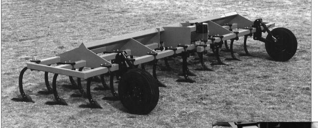
*The Bigham Chisel Plow (8" or 12" Space)* allows shank spacing on 8" or 12" centers. Shanks spaced on 8" centers with sweeps allow use of chisel plow as a field conditioner. The closer shank spacing reduces the ridging effect of sweeps.
