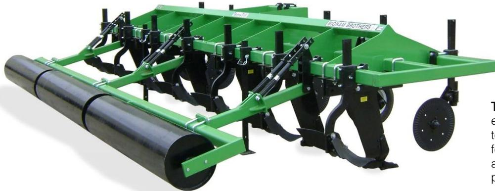
TerraTill® above is equipped with bedding tools and bed rollers for a one pass tillage and seedbed preparation tool.
