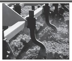
attachment may be adjusted to operate rod at anticipated planting depth. Rod seals moisture at operating depth so that seed may be placed in fresh, moist soil.
