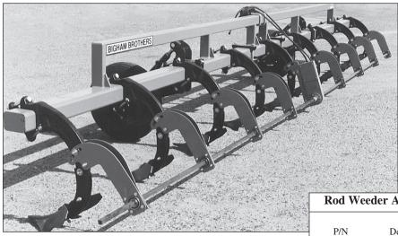
Remove weeds and condition seedbeds behind your High Clearance Lister with the Bigham Brothers Hydraulic Center Drive Rod Weeder specifically designed for the high clearance lister beam. This attachment will knock the top of the bed down, seal moisture at a consistent depth and condition the very top of the bed to act as an abrasive when you follow with a planter equipped with double disc openers.
