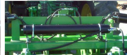
Optional Accumulator is required for most applications.
