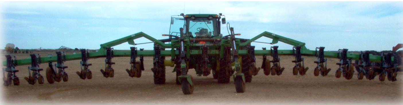
Stack Fold Tool Bars are designed for tractors up to 250 HP. Specifications are for standard Stack Fold tool bars.
