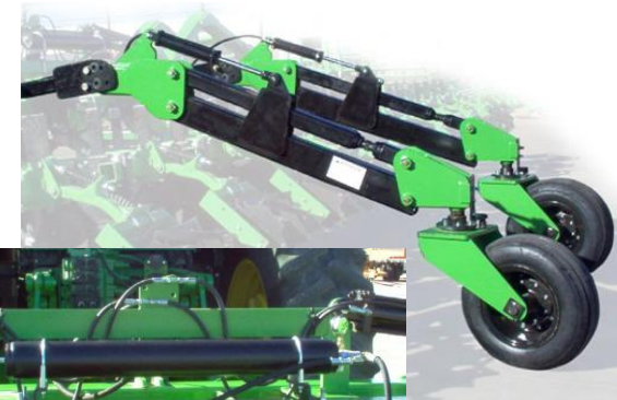
Patented Stack Lock® transport lock joint
