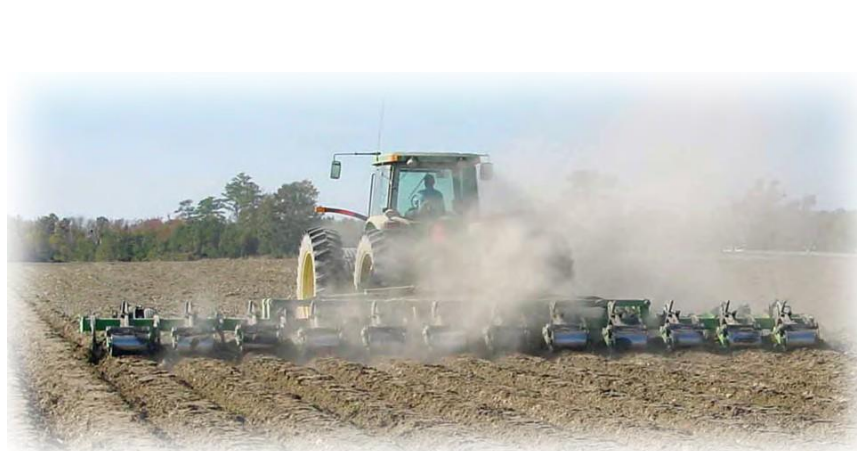
Bedder Tool Bar with lister beams and rollers.
